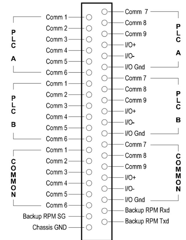
By observing certain X points, each PLC can determine whether it is the active or the standby controller and whether the other PLC is available for transfer of control. If a dual-RPM architecture is used, the status of the backup RPM module can also be monitored. Y control points can be used to request a switchover to the other PLC, or to the backup RPM (if present).
