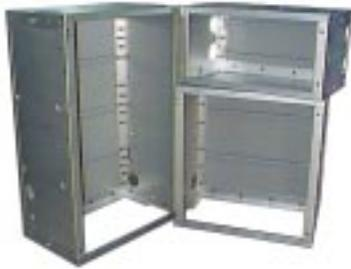
The ABB design concept for metal-clad switchgear is to locate protection and control devices in dedicated low voltage (LV) compartments. This completely isolates and segregates control equipment and circuits from high voltage areas, providing maximum safety for operations and maintenance personnel working on switchgear controls.
