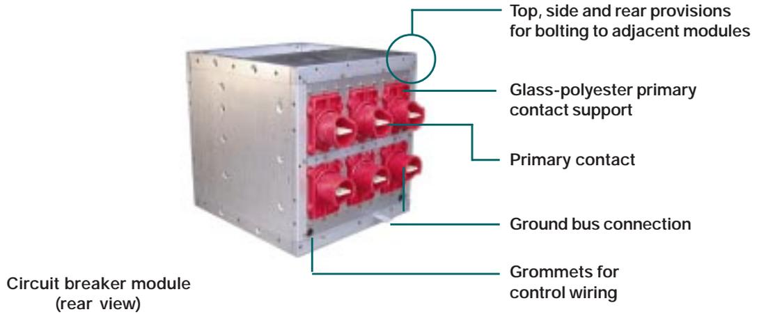
Each module has bolt provisions for connection to upper or lower modules in the same vertical section, connection to modules in adjacent vertical sections, and attachment of primary bus barriers and rear cable compartments fabricated by the switchgear assembler.
